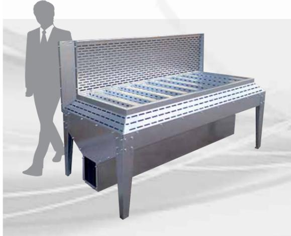
Galvanized sheet workbench with suction from the bottom, from the sides and from the front, to carry out sanding operations in total safety thanks to the suction slots on the work top, covered with scratch-resistant felt (optional). Available in different sizes (customized solutions are possible), it requires a connection to a central suction system.
