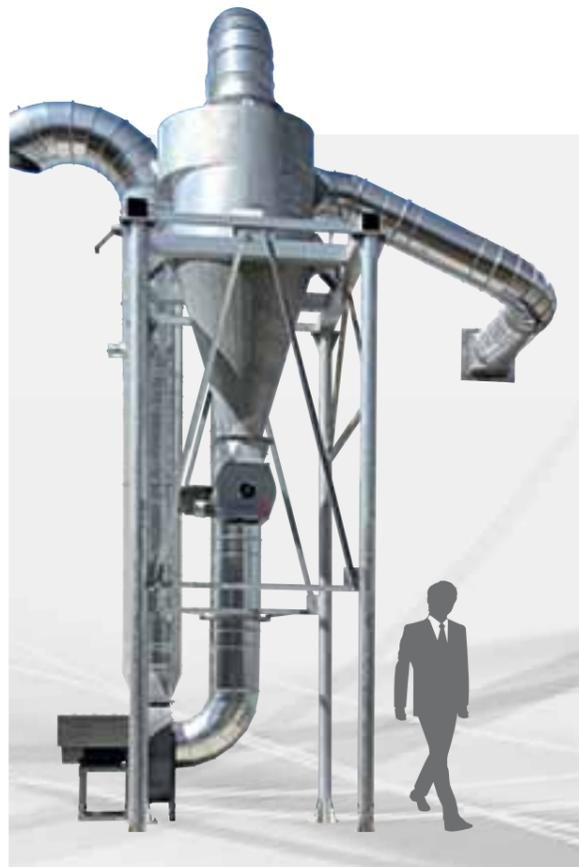
Centrifugal dedusting separator, made of galvanized steel, suitable for the filtration of medium-large particles. Dedusting of the powders takes place by effect of the centrifugal force caused by the spiral motion imposed on the treated fluid during the passage inside the separator.
