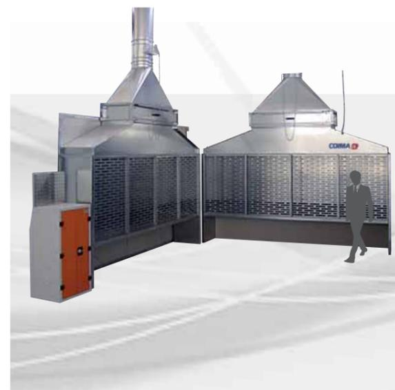
Wall made of slotted galvanized sheet metal, with customised shape and size, ideal to immediately remove the fumes produced by welding operations on large surfaces from the operator; it is equally suitable to suck up dust clouds produced by grinding/sanding operations.
